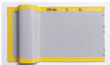
Figure 21. Test panel after humidity 1000 hours
