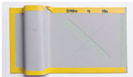
Figure 21. Test panel after humidity 1000 hours
