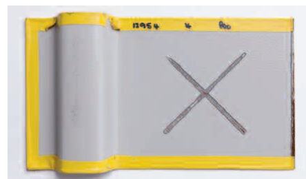
Figure 22. Test panel after Watersoak 1000 hours
