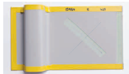
Figure 22. Test panel after Watersoak 1000 hours
