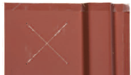
Figure 18. Test panel after water soak 1000 hrs
