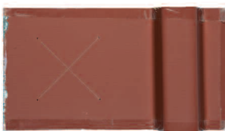
Figure 15. Test panel after saltspray 1000 hrs
