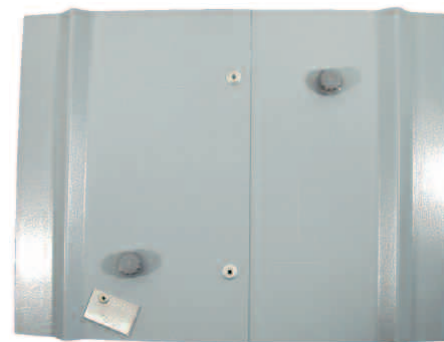
Figure 12. A Colorcoat Prisma® test panel after more than 2 years exposure
