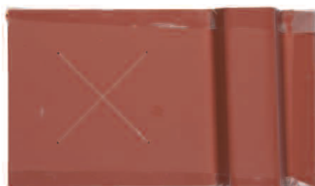
Figure 17. Test panel after humidity 1000 hrs
