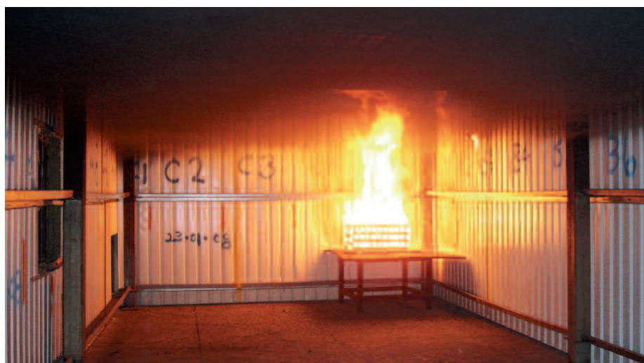
Figure 28. Example of material during an LPS 1181 test
