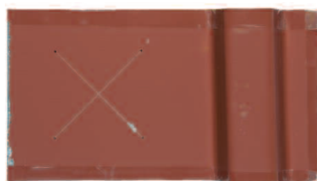
Figure 16. Test panel after prohesion 1000 hrs
